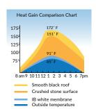
A white IB Roof Systems membrane can reduce your energy consumption and your rising electric bills, by reflecting up to 90% of the heat that normally enters a building through the roof. An IB Roof Systems roof will lower your building's heat gain, and possibly pay for itself.
