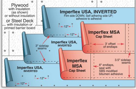
**IMPERFLEX** Roof Systems should not be installed directly over a wood plank deck without a layer of roof insulation and/or Dens-Deck or other approved barrier board.
